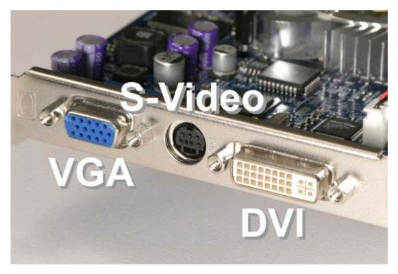
Most new desktop computers include two connectors to support dual monitors.
